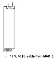
Prepared power cable for voltage input and cables for connection of the automaton outputs (connection of the electrical lock with the automaton, connection of the other outputs used)
